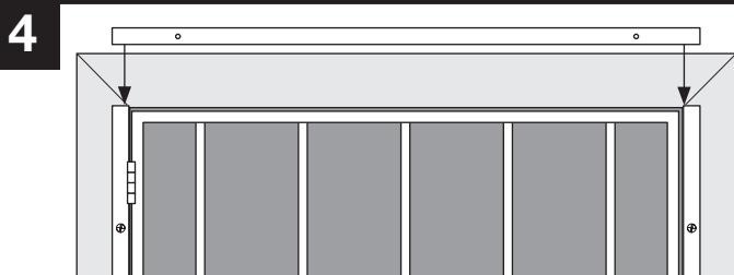
Position the top header jamb (C) across the top of the two side jambs. Make certain there is a minimum 1/8" space between the header and the top of the door frame, and that the header is level.
